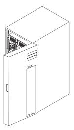
2. Loosen the retained screws that hold the disk drive cover to the drawer and remove the disk drive cover from the drawer, storing it in a safe place.
